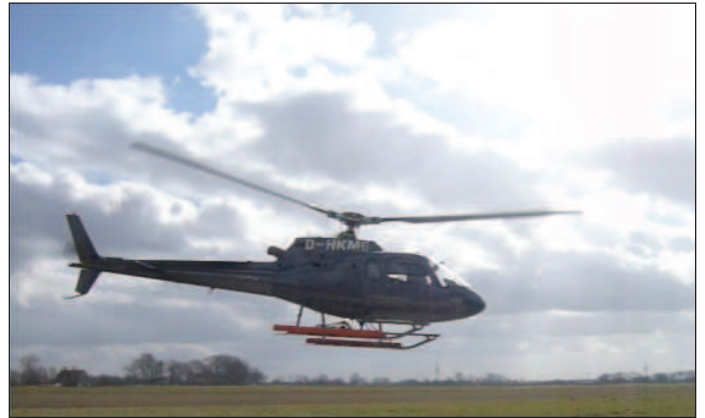
Figure 3: Continuously measurements of time-varying component of natural EM field by slow and low helicopter flights along survey lines
